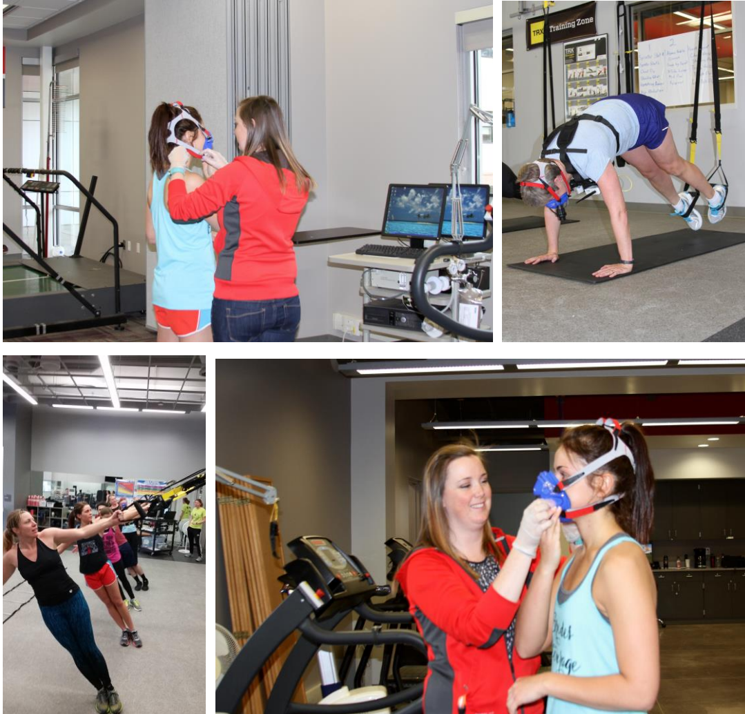
Figure 1. – The Oxycon Mobile metabolic system attached to a participant before (upper left & lower right) and during (upper right & lower left) a TRX Suspension Training class.
